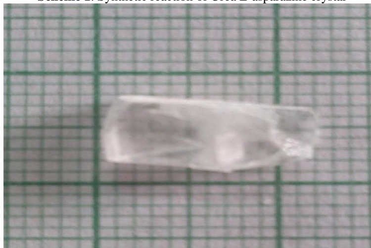
Photograph of as grown single crystals of urea L-asparagine
